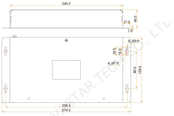
Tolerance: ±0.3 Unit: mm
